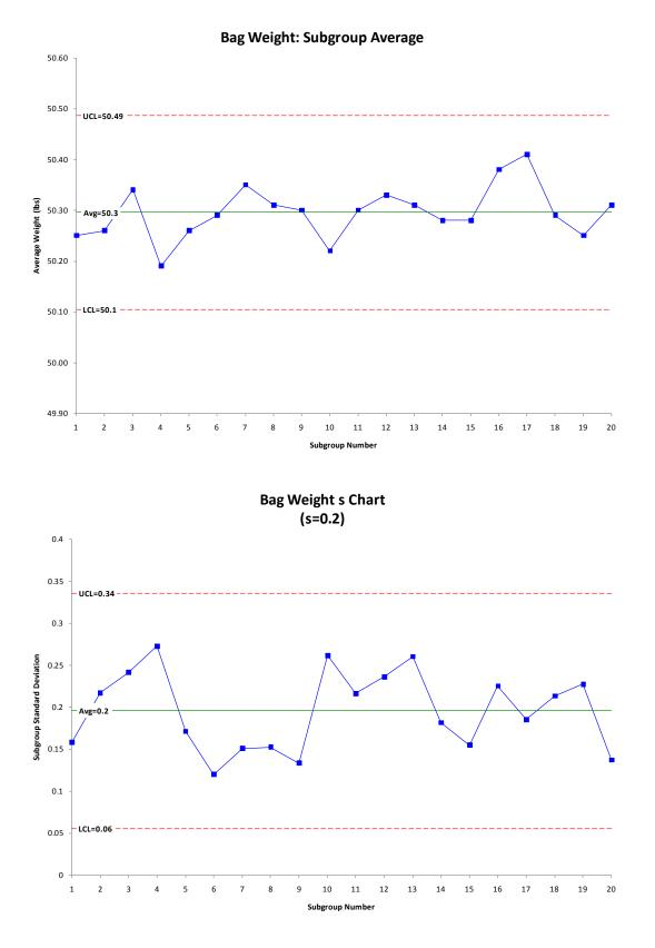
Figure 1: Bag Weight  $\overline{X}$  -s Control Chart
